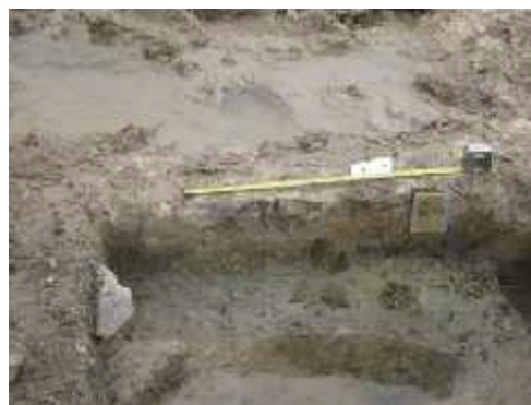
Fig. 4: Detail of Sample 652 through light grey (10YR6/1) 'white layer' and an underlying reddish yellow (7.5YR6/8) layer. Whitish material can be found within the dominantly dark grey and grey (5Y4/1-5/1) clay substrate (weathered Permo-Triassic mudstone).
