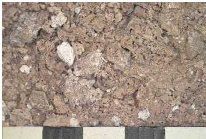
Plate 3: The calcareous tufa residue from the partial dissolution of a sample from 623. Fragments of undissolved white lime can also be seen.
