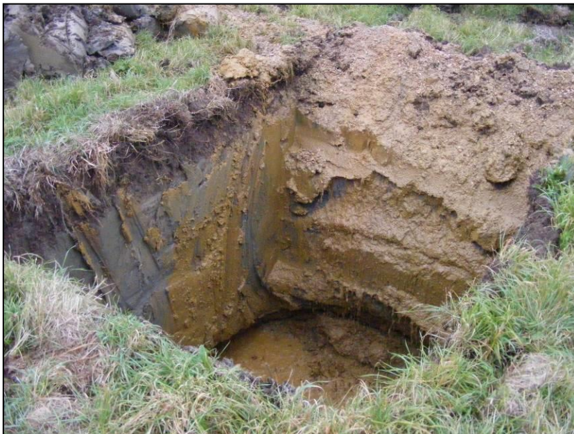
Left: Test-pit B, showing the deep alluvium and exposing the underlying gravels.
