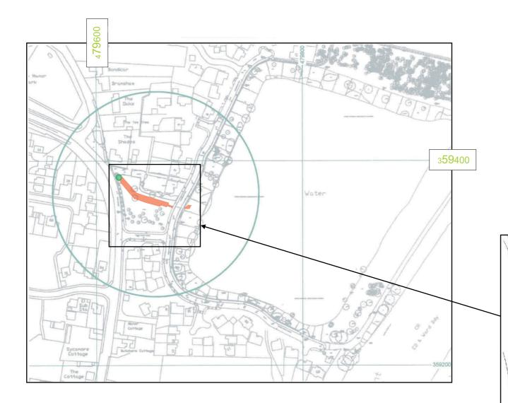
**Fig.2:** General Site Location at Scale 1:2500 (above). The area of hand excavation is shaded green, and the area stripped for the pipe trench easement is shaded in red.
