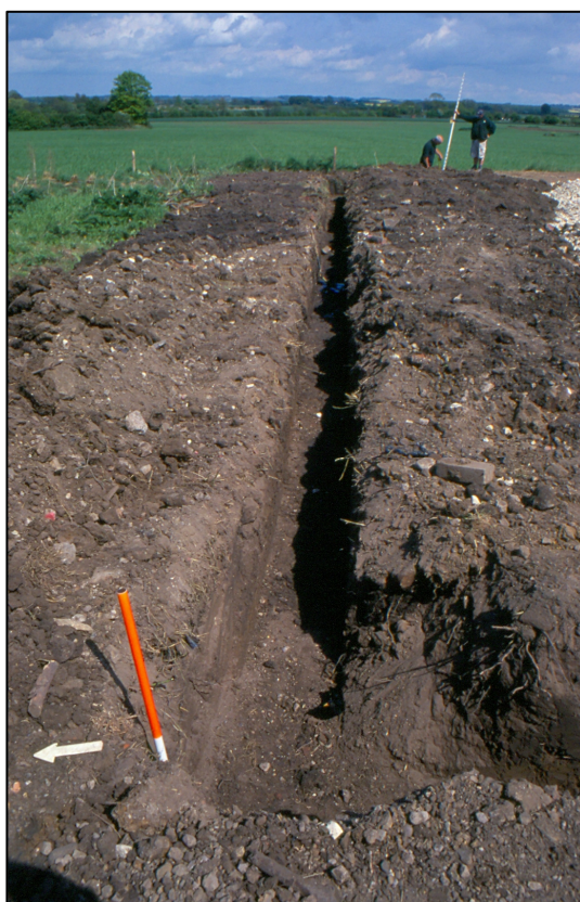
Pl. 12 To the south of the house, a percolation test pit encountered thick imported rubble directly above weathered boulder-clay natural. Scale 1m).
