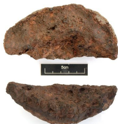
Figure F.1. Plano-convex dense iron silicate (DIS) recovered from context [20008]
