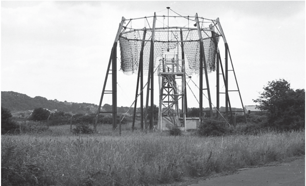
Plate 21: Believed to be the short-range transport rig, September 1982. Note the torpedo netting to contain an engine or rotor failure.
