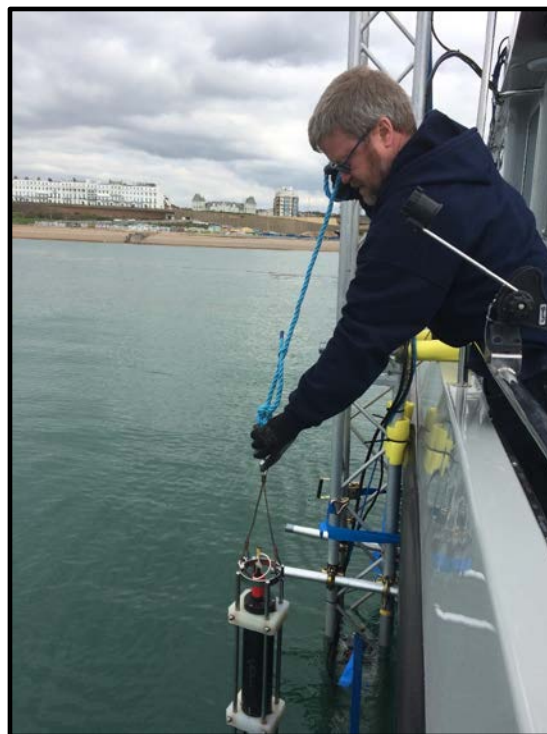
Figure 4: Preparing to take a sound velocity profile
