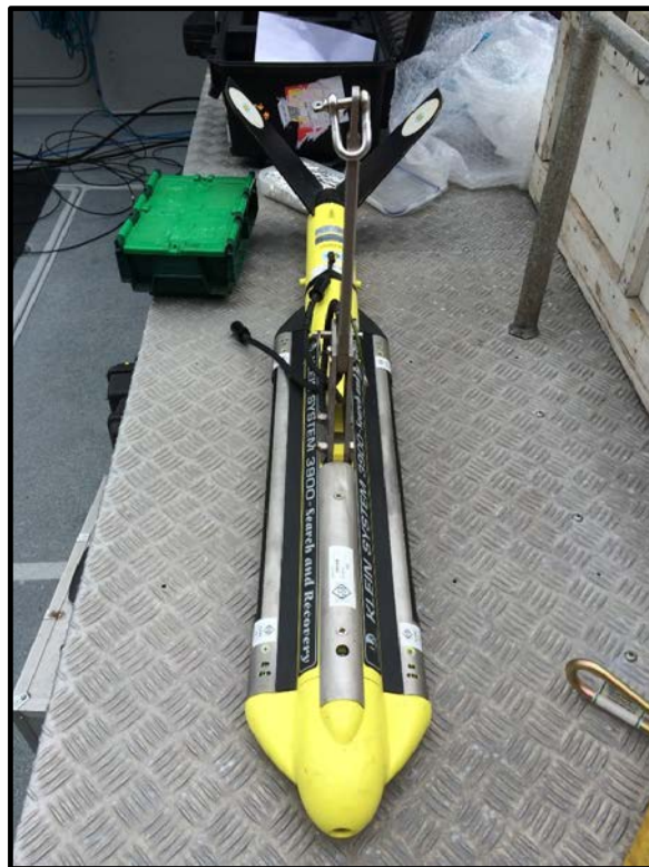
Figure 6: Klein 3900 sidescan sonar
