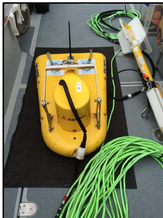
Figure 5: EdgeTech SB-216S towfish
