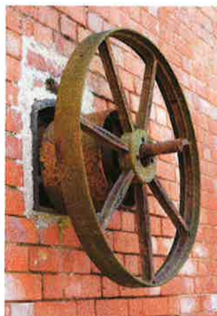
Pl.38: The belt wheel attached to the shafting in the Barn close to the 'cut-out'.
