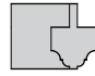
Profile of original stiles of sashes in F1 (glazing bar profile inset)
