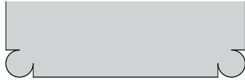
Profile of architrave to arched openings between F3, and F5 and F6
