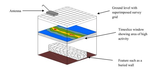
The GPR data is compiled to create a 3D file. This 3D file can be manipulated to view the data from any angle and at any depth within a range. The 3D file can be sampled to produce activity plots at various depths. As the radar is actually measuring the time for each of the reflections found, these are called "time slice windows". Plots for various time slices have been included in the report. Based on an average velocity calculations have been made to show the equivalent depth into the ground.
