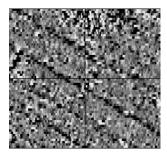
Ploughing activity can often be visualised by a series of parallel linear anomalies. These can be of either positive polarity or negative polarity depending on site specifics. It can be difficult to distinguish between ancient ploughing and more modern ploughing. Clues such as the separation of each linear, straightness, strength of response and cross cutting relationships can be used to aid this, although none of these can be guaranteed to differentiate between different phases of activity.
