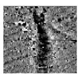
Weakly magnetic wide scale variations within the data can sometimes be seen within sites. These usually have no specific structure but can often appear curvy and sinuous in form. They are likely to be the result of natural features, such as soil creep, dried up (or seasonal) streams. They can also be caused by changes in the underlying geology or soil type which may contain unpredictable distributions of magnetic minerals, and are usually apparent in several locations across a site.
