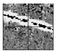
A positive linear anomaly which has a negative anomaly located adjacently. This will be caused by a single feature. In the example shown this is likely to be a single length of wire/cable probably relating to a modern service. Magnetically weaker responses may relate to earthwork style features and field boundaries.
