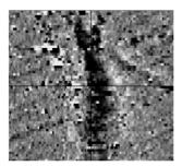
Weakly magnetic wide scale variations within the data can sometimes be seen within sites. These usually have no specific structure but can often appear curvy and sinuous in form. They are likely to be the result of natural features, such as soil creep, dried up (or seasonal) streams. They can also be caused by changes in the underlying geology or soil type which may contain unpredictable distributions of magnetic minerals, and are usually apparent in several locations across a site.
