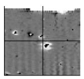
This consists of a single positive anomaly with an associated negative response. There should be no separation between the two polarities of response. These responses will be created by a single feature. The interpretation of the anomaly will depend on the magnitude of the magnetic measurements. A very strong anomaly is likely to be caused by a ferrous object.
