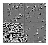
Magnetic debris consists of numerous dipolar responses spread over an area. If the amplitude of response is low (+/-3nT) then the origin is likely to represent general ground disturbance with no clear cause, it may be related to something as simple as an area of dug or mixed earth. A stronger anomaly (+/-250nT) is more indicative of a spread of ferrous debris. Moderately strong anomalies may be the result of a spread of thermoremanent material such as bricks or ash.
