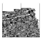
A linear response which is entirely negative in polarity. These are generally caused by earthen banks where material with a lower magnetic magnitude relative to the background top soil is built up. See also ploughing activity.
