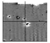
This consists of a single positive anomaly with an associated negative response. There should be no separation between the two polarities of response. These responses will be created by a single feature. The interpretation of the anomaly will depend on the magnitude of the magnetic measurements. A very strong anomaly is likely to be caused by a ferrous object.
