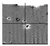
This consists of a single positive anomaly with an associated negative response. There should be no separation between the two polarities of response. These responses will be created by a single feature. The interpretation of the anomaly will depend on the magnitude of the magnetic measurements. A very strong anomaly is likely to be caused by a ferrous object.
