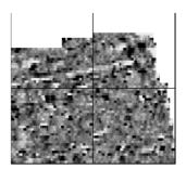
A linear response which is entirely negative in polarity. These are generally caused by earthen banks where material with a lower magnetic magnitude relative to the background top soil is built up. See also ploughing activity.
