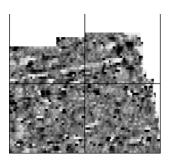
A linear response which is entirely negative in polarity. These are generally caused by earthen banks where material with a lower magnetic magnitude relative the background top soil is built up. See also ploughing activity.
