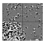
Magnetic debris consists of numerous dipolar responses spread over an area. If the amplitude of response is low (+/-3nT) then the origin is likely to represent general ground disturbance with no clear cause, it may be related to something as simple as an area of dug or mixed earth. A stronger anomaly (+/-250nT) is more indicative of a spread of ferrous debris. Moderately strong anomalies may be the result of a spread of thermoremnant remnant material such as bricks or ash.
