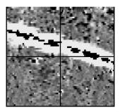
A positive linear anomaly which has a negative anomaly located adjacently. This will be caused by a single feature. In the example shown this is likely to be a single length of wire/cable probably relating to a modern service. Magnetically weaker responses may relate to earthwork style features and field boundaries.
