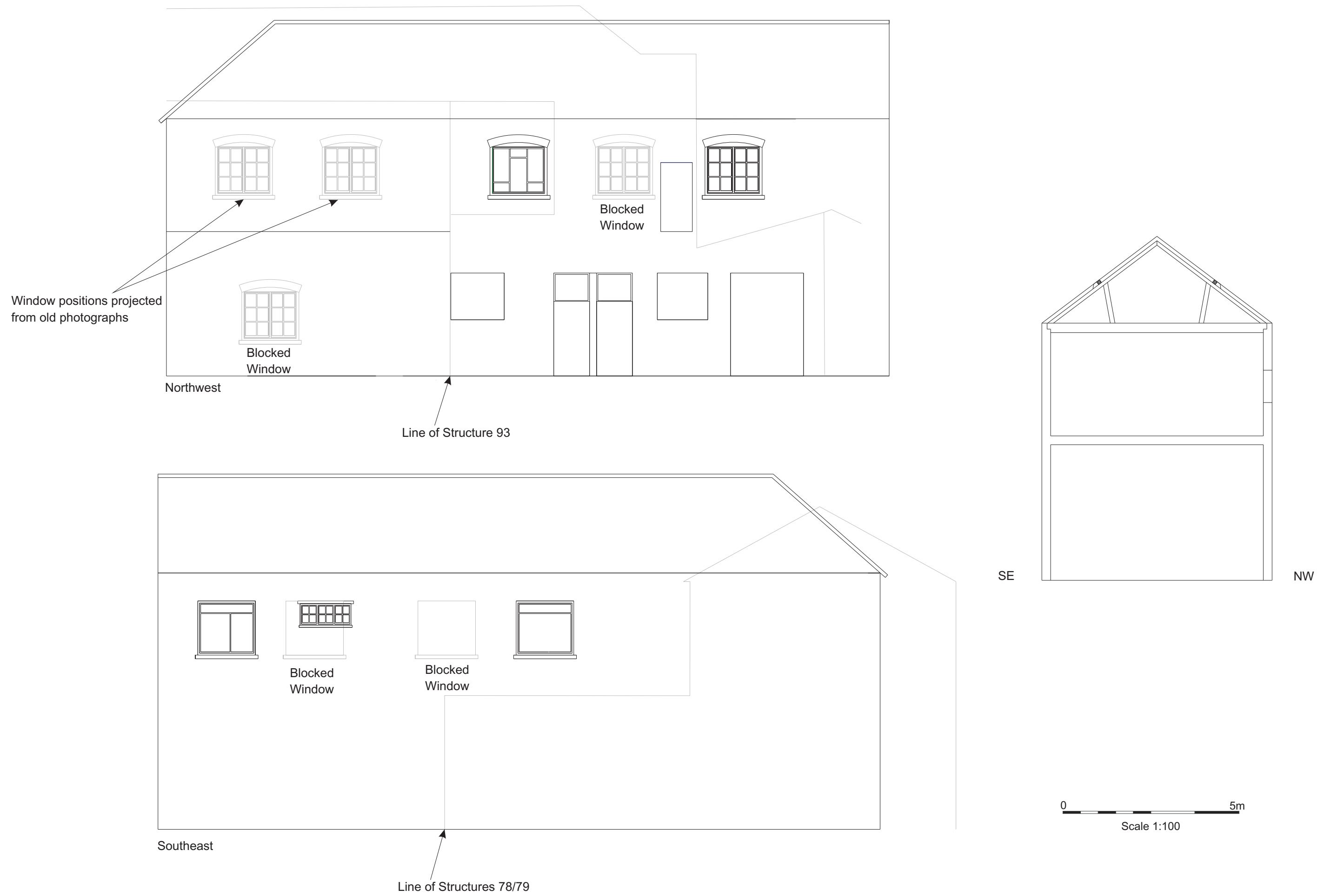
Figure 100: Structure 48 (The Down Room) Elevations and Cross-Section
