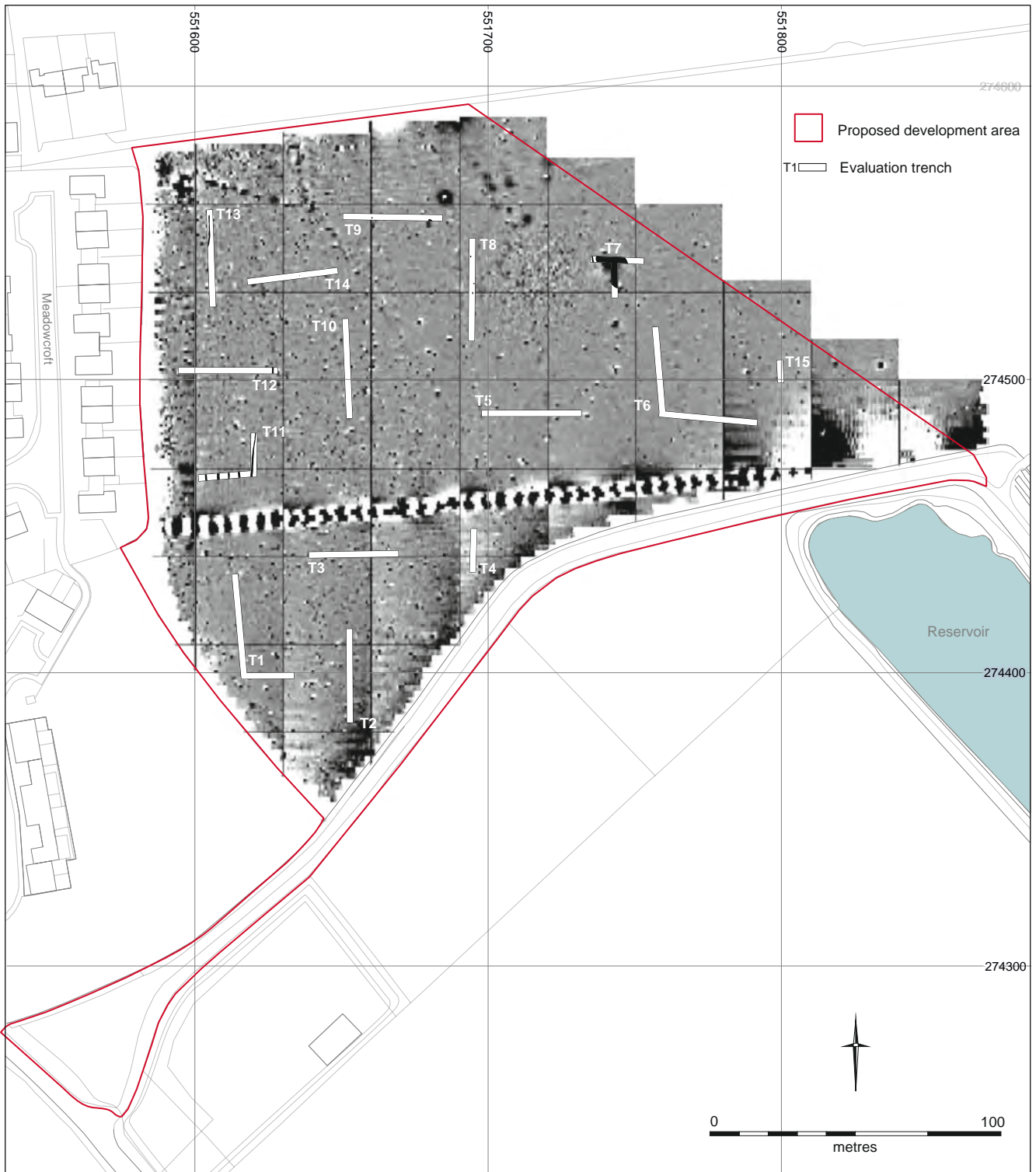
Figure 2. Trench plan with geophysical survey results
