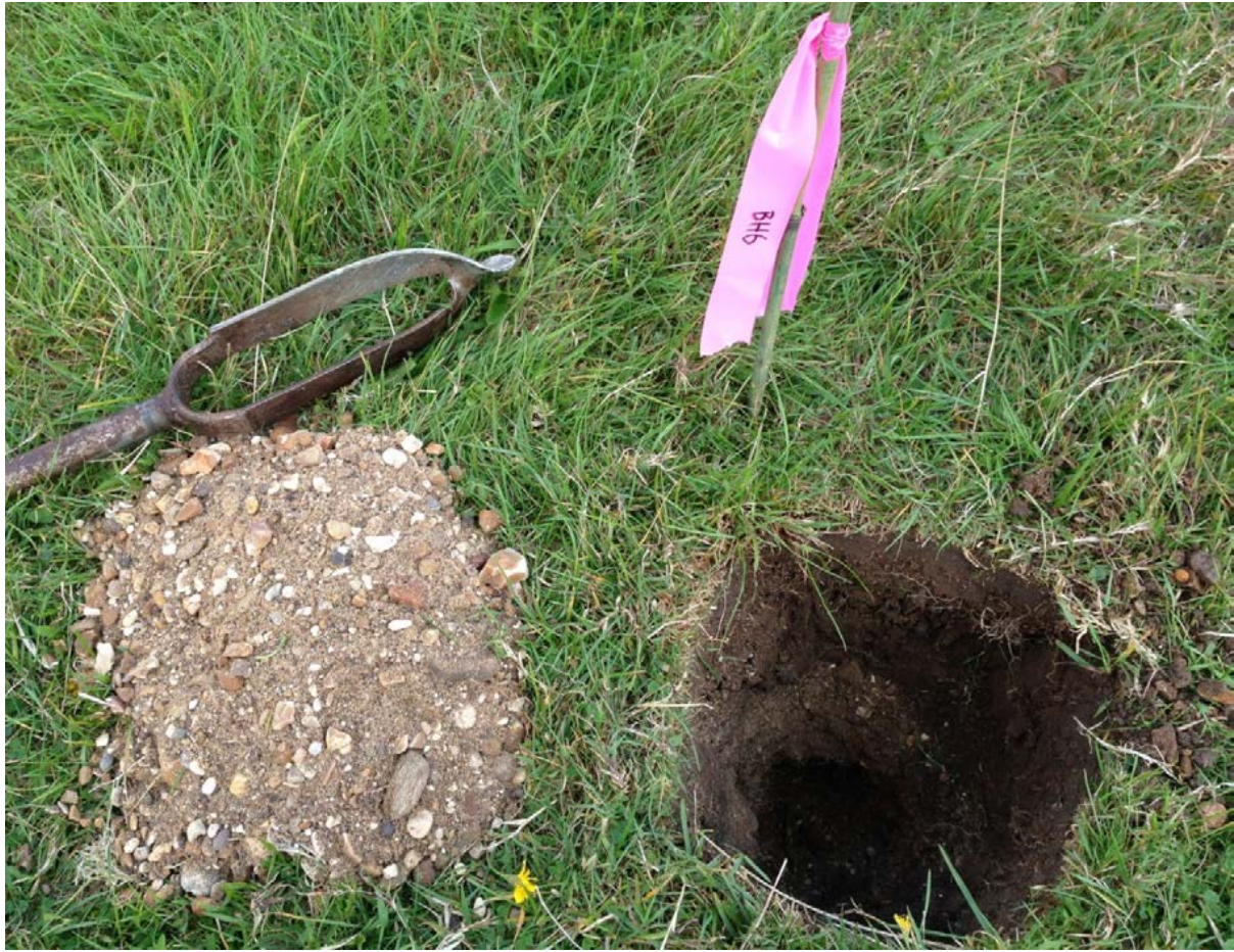
Figure 11. Field photograph of gravel obtained from BH6 at 25 – 50cm below the surface.
