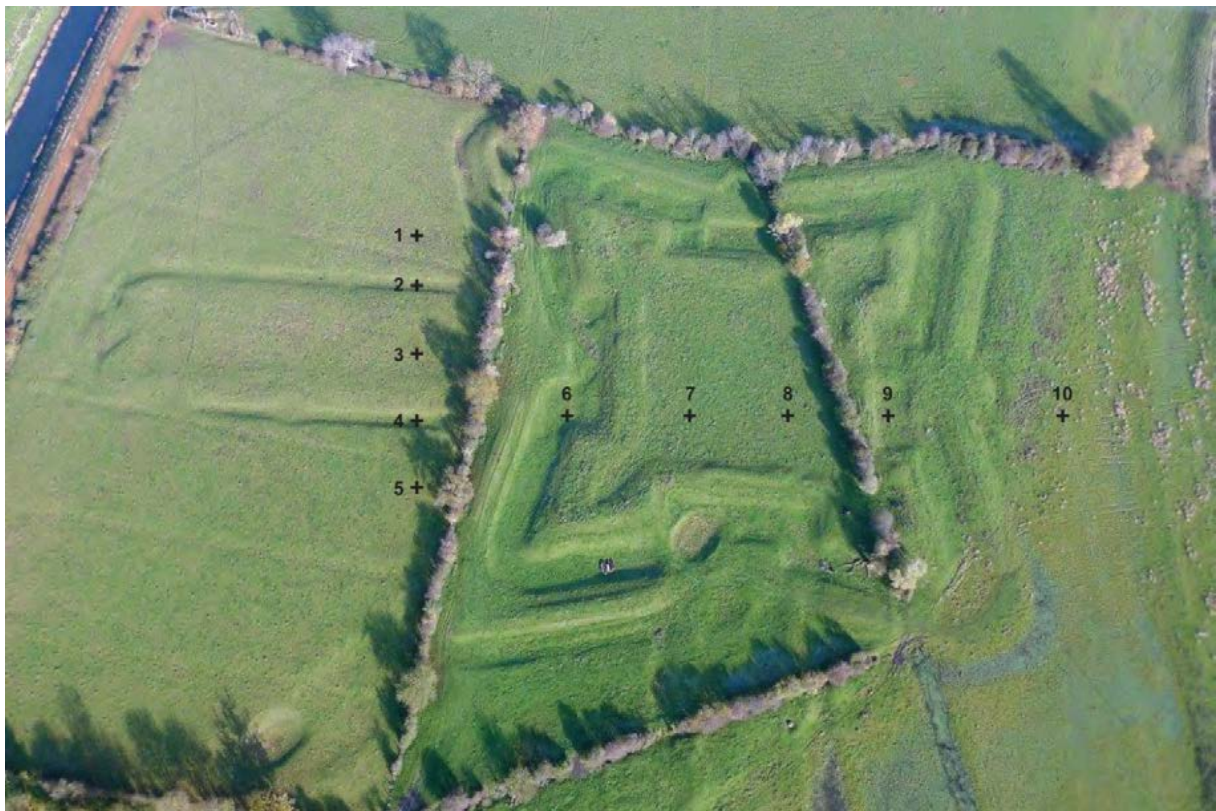
Figure 10. Aerial photograph of Earith Bulwark, showing the location of boreholes BH1-10 arranged in two transects T1 (N-S BH1-5) & T2 (W-E BH6-10).
