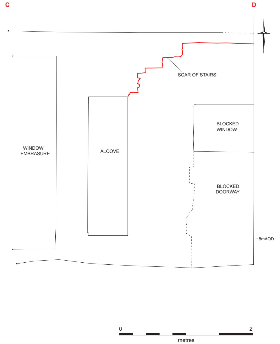
Figure 8. Partial elevation of the east wall of the Porter's Lodge, with photograph (facing east) and drawing highlighting principal build elements
