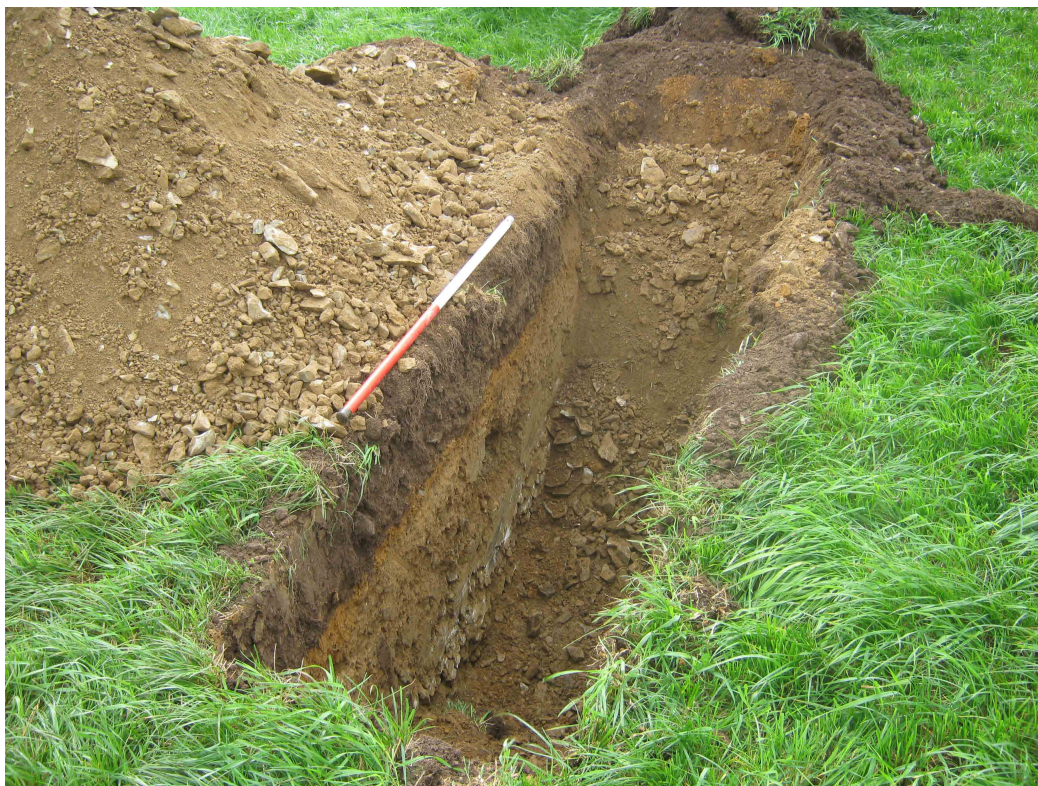
Fig.4 - Oblique shot of the section of completed trial pit TPT4D
