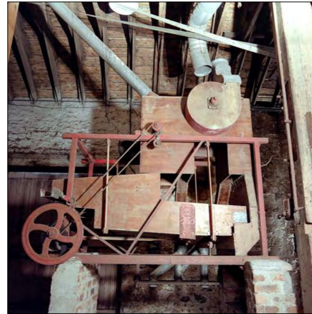
Plate 50 - Range A, Detail on the grain feeder, built by Boswell's of Blairgowrie.
