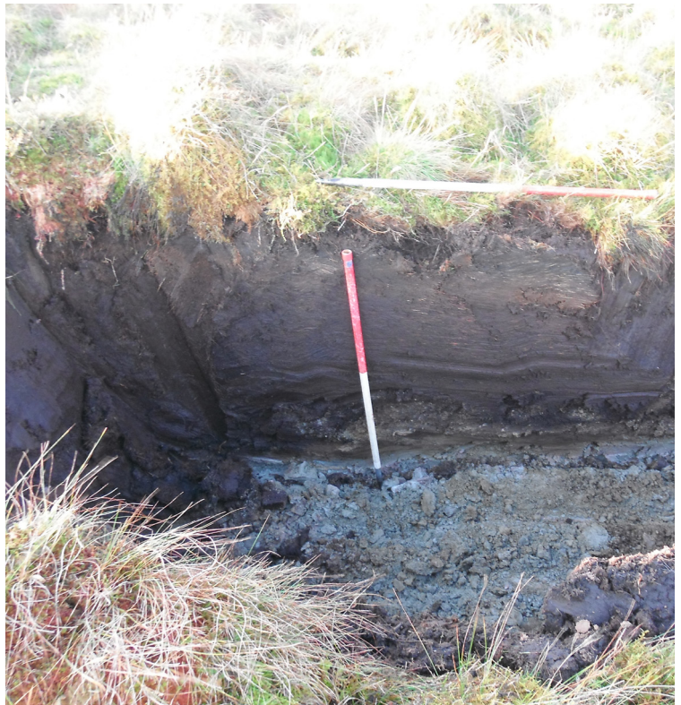
Fig. 20 - Trial Pit 081 showing peat section
