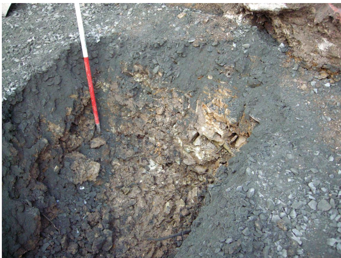
Plate 2 - Test Pit 1 and exposed sandstone bedrock close to ground level
