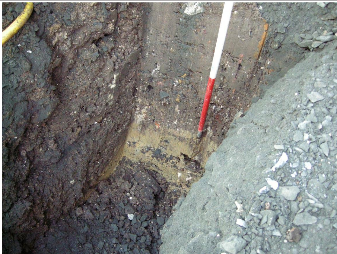
Plate 3 - Test Pit 2 showing the depth of natural clay approximately 0.9m below ground level
