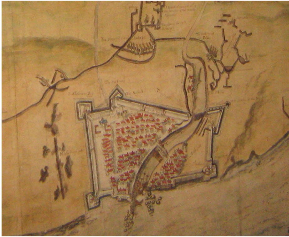
Fig. 7 Detail of the Petworth Map, 1560, showing the Italian style defensive works built around Leith
