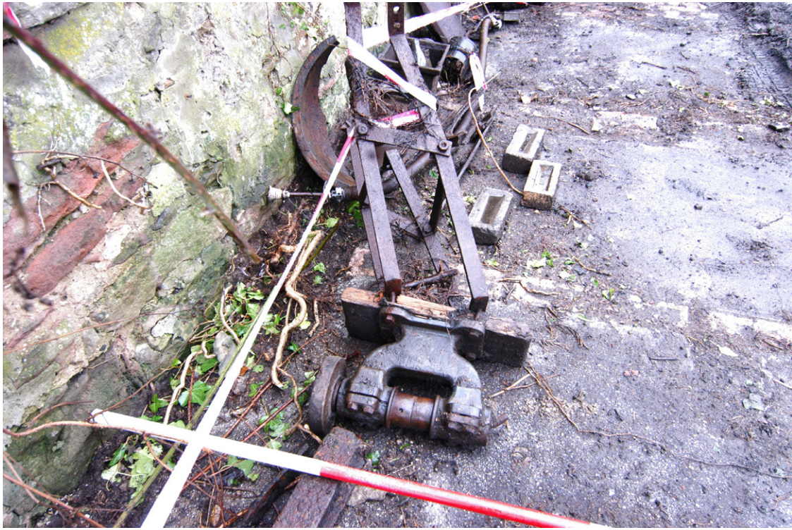
Fig. 12 A belt-driven grinding stone found during site clearance
