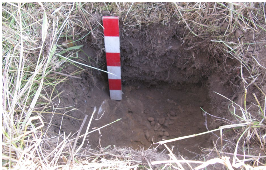
Fig. 3 - Starter pit for borehole 3.1a
