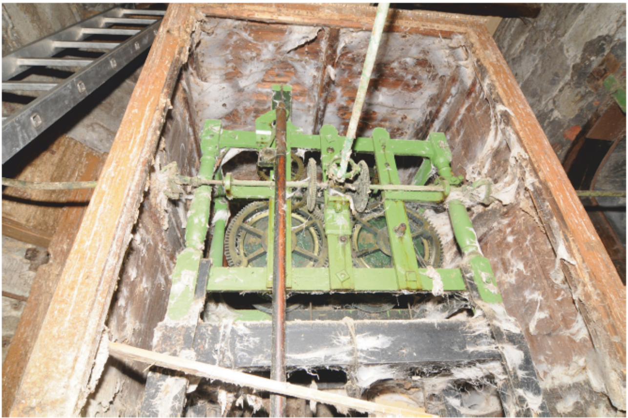
Fig. 31 - The clock mechanism housed at the top of the weight chamber
