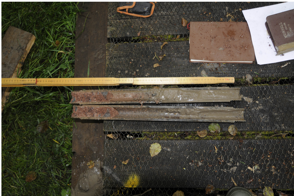
Fig. 7 - Fractured bedrock exposed in the SPT sampler barrel at -3.6m
