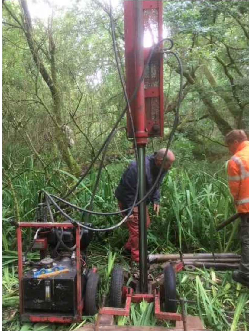
Fig. 2 - Competitor Dart Percussion Rig used to take borehole window samples
