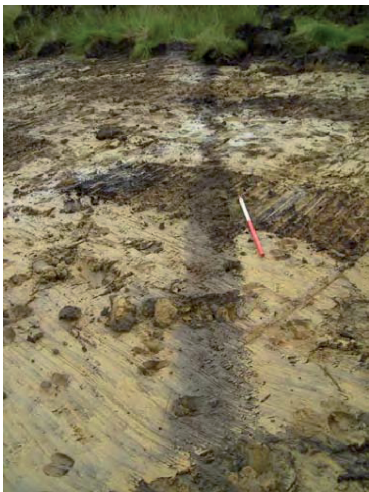
Fig 28. Drainage ditch 085 in plan
