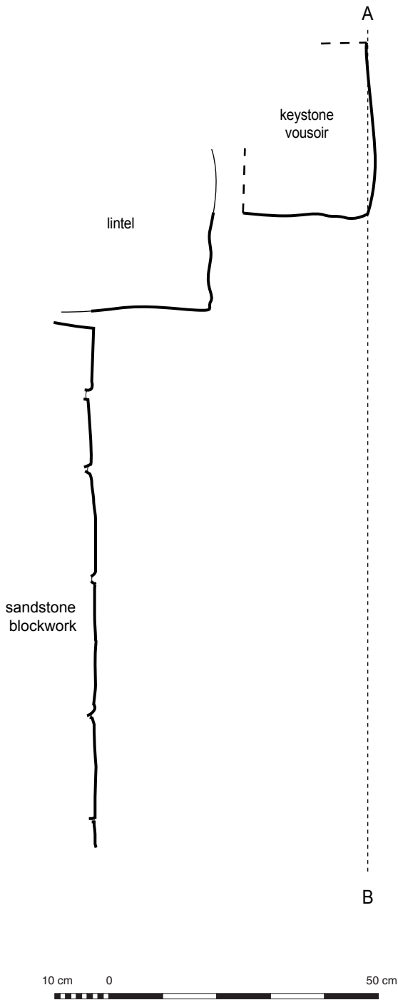
Fig. 25a - Profile of basement door with blocking in place
