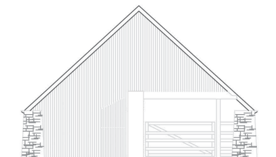
Fig 3c. Existing East Elevation before the timber cladding was removed
