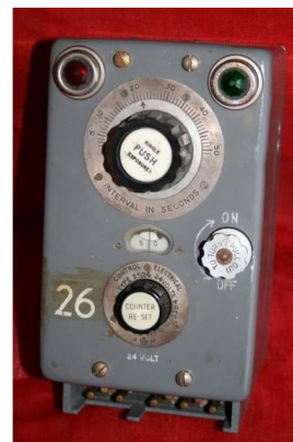
Figure 13, Undamaged control unit.
