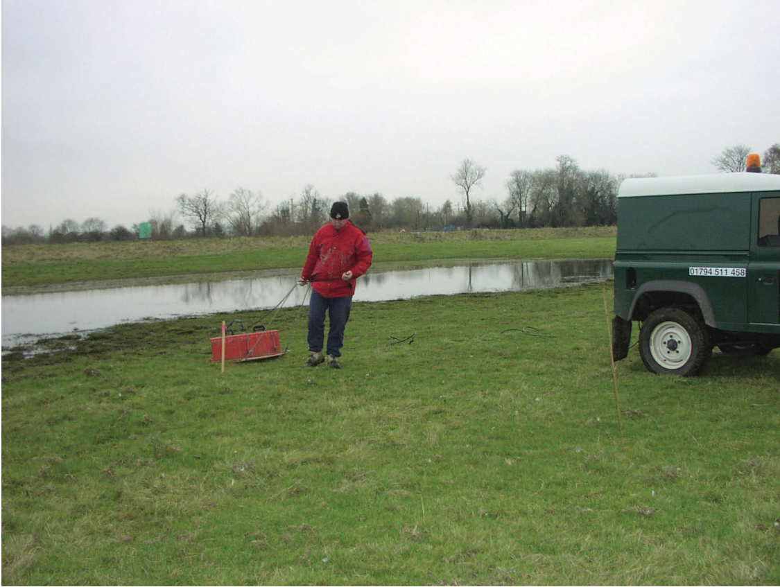
Fig 3.2: The GPR survey about to start on the modern floodplain, using a 200MHz antenna.
