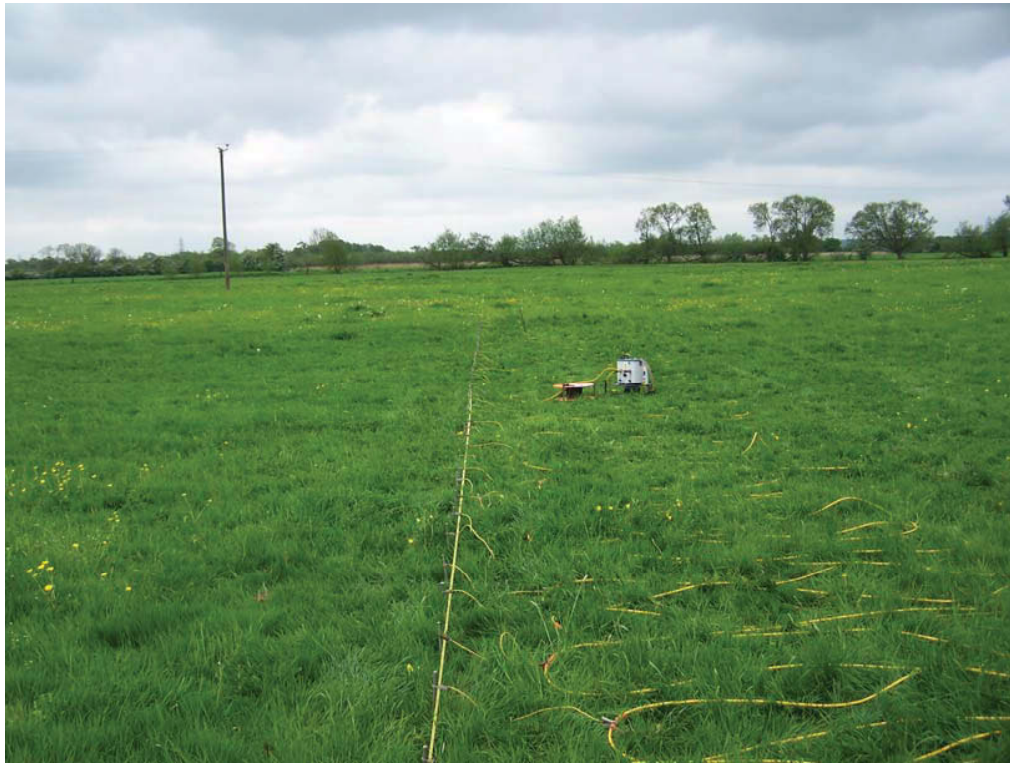
Fig 3.16: ER transect running across a palaeochannel on the lower floodplain. The IRIS Junior unit is central between the two cables. Each cable is attached to 24 electrodes.
