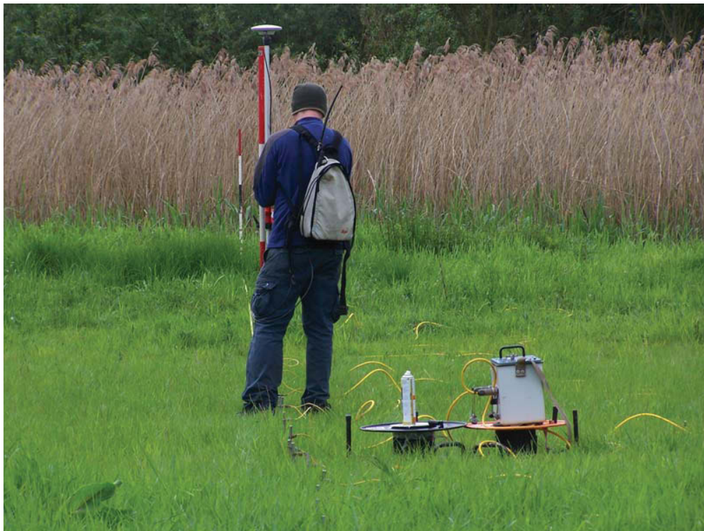
Fig 3.17: Recording the position of the ER transect T1F using dGPS.
