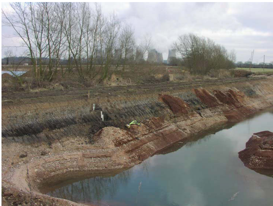
Fig 3.7: Palaeochannel WFQ C2 during sampling, with the tins in-situ before removal. The stratigraphy drawn in the section of red-brown silty clay above a grey silty clay, above a dark grey silty clay is clearly visible.
