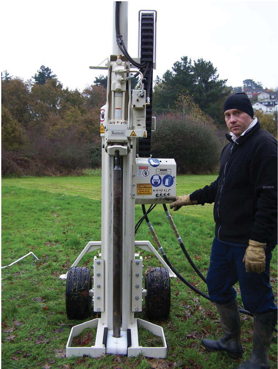
Fig 3.1: The Geoprobe coring rig, about to commence a drive. The closed metal chamber is seen at the front of the rig, with a plastic sample collection tube located within it.
