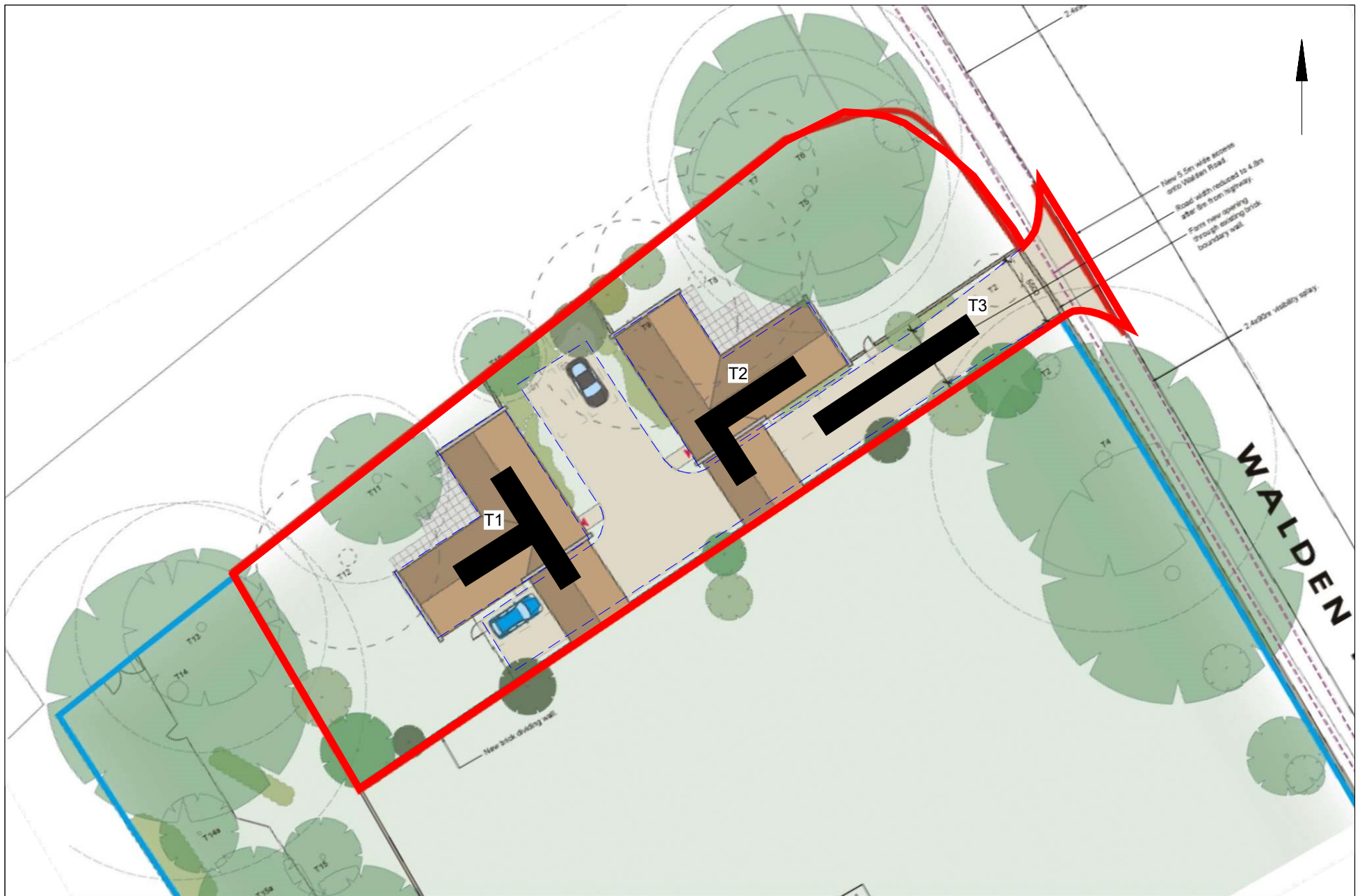
Fig 2 Trench layout in relation to proposed development (dashed blue lines) and arboreal constraints.
