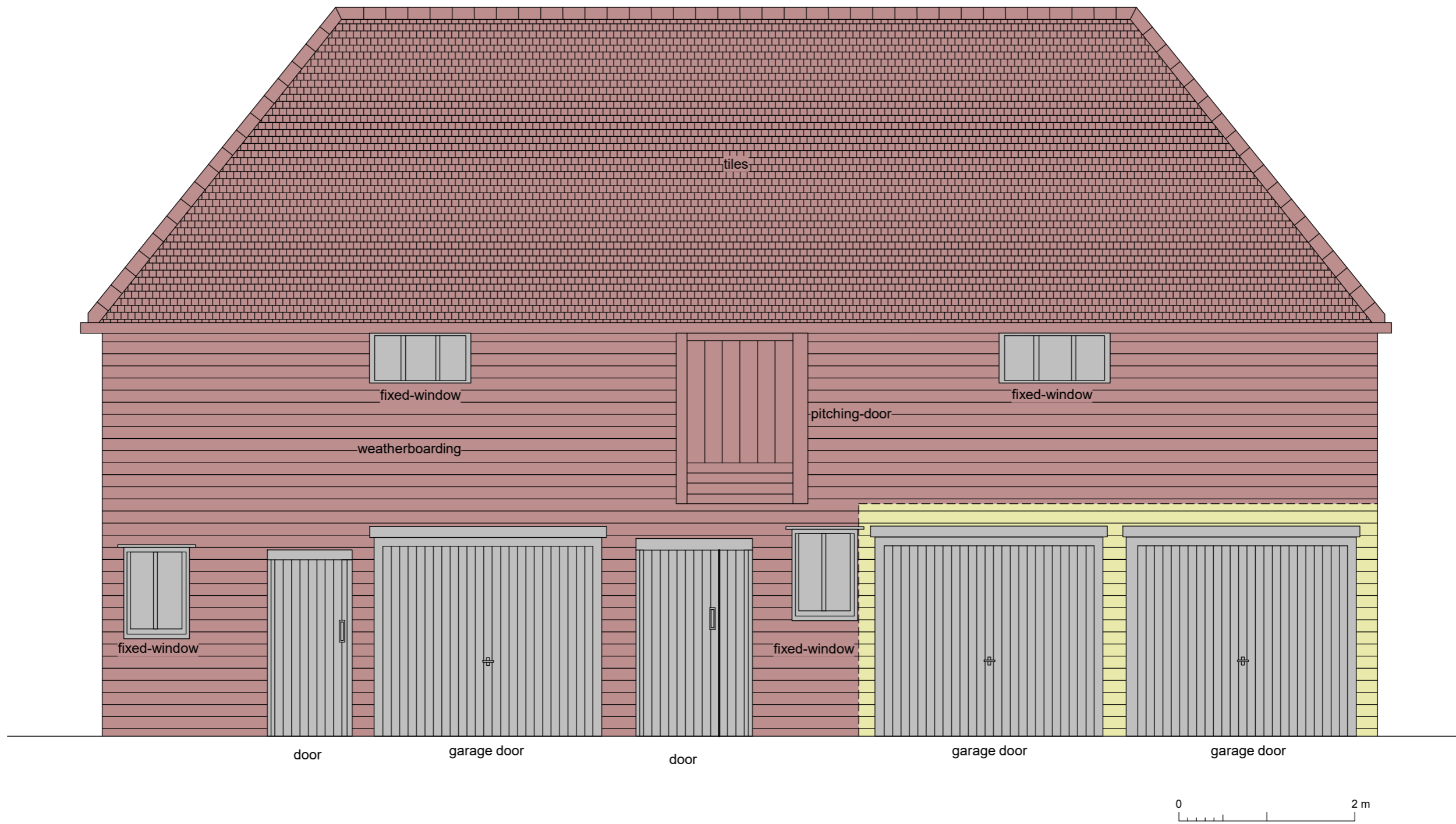
Fig 4 Southern elevation of building, with phasing (phasing shows dates of the structural elements, not the weatherboarding).
