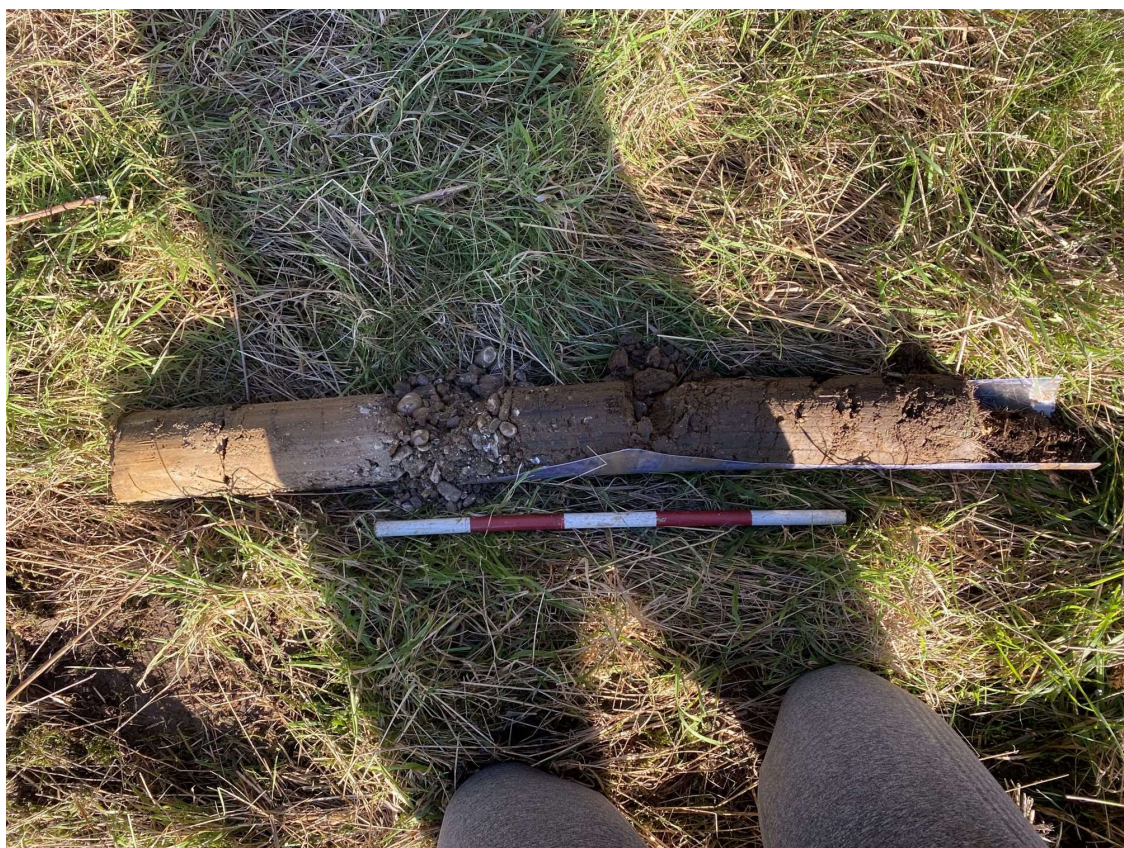
Photograph 5 WS1 core (0-1m)
