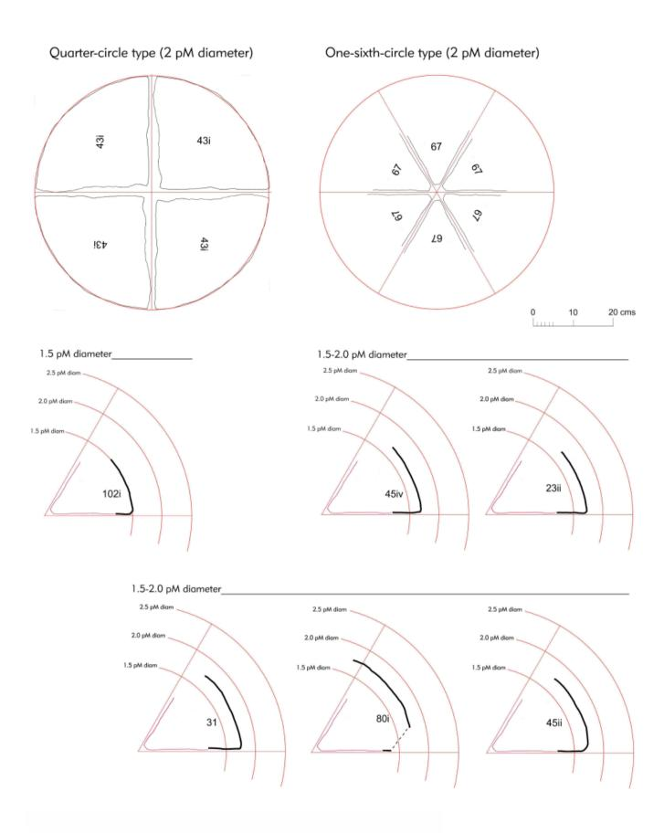
Fig 16 Analysis of the Roman column brick in terms of radii: sheet 1.
