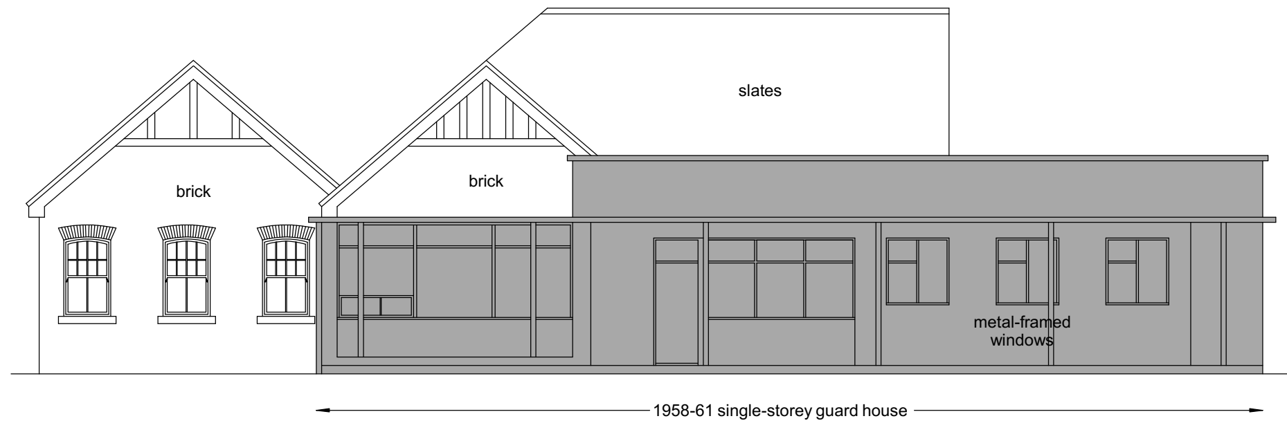
Fig 25 MEE 01: south elevation of the former Meeanee Barracks Brigade Offices, with alterations shaded grey.
