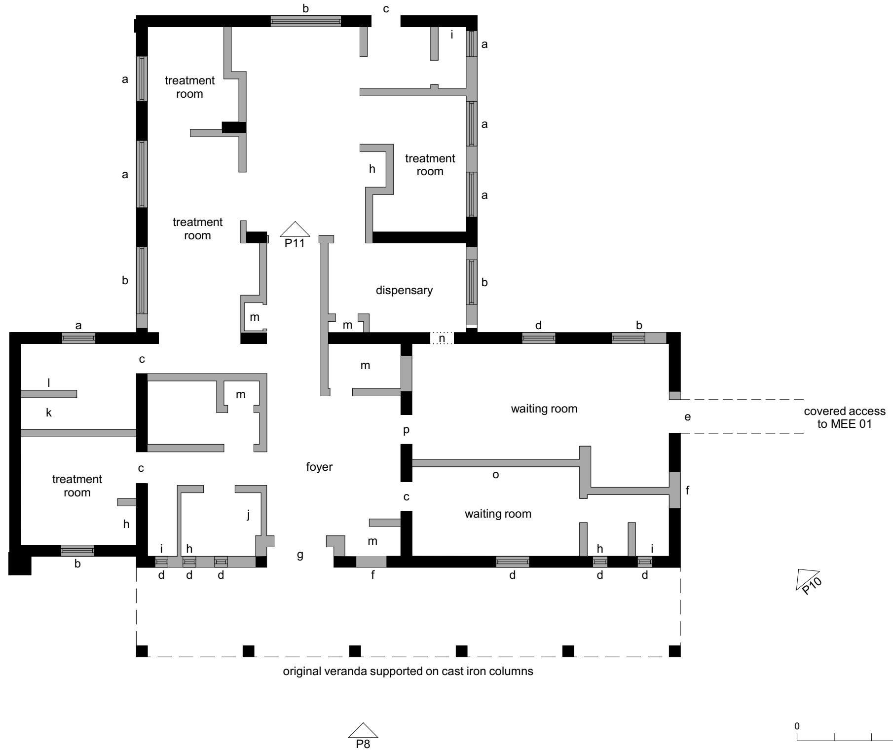
Fig 29 MEE 03: floor plan of the former Meeanee Barracks Guard House, with original fabric shown black and medical centre alterations shaded grey. The location and orientation of photographs included in this report are indicated by the numbered arrows.
