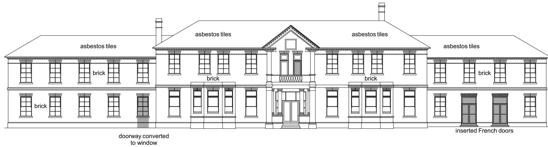
Fig 43 HYD 08: west elevation of the Hyderabad Barracks Officers' Mess and Quarters, with alterations shaded grey.
