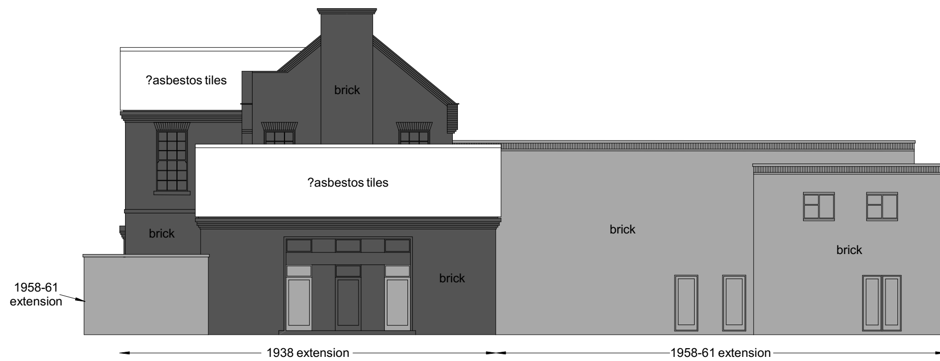
Fig 52 HYD 11: west elevation of the Hyderabad Barracks Regimental Institute, with alterations shaded grey.
