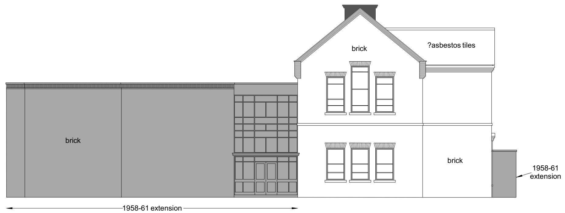
Fig 50 HYD 11: east elevation of the Hyderabad Barracks Regimental Institute, with alterations shaded grey.
