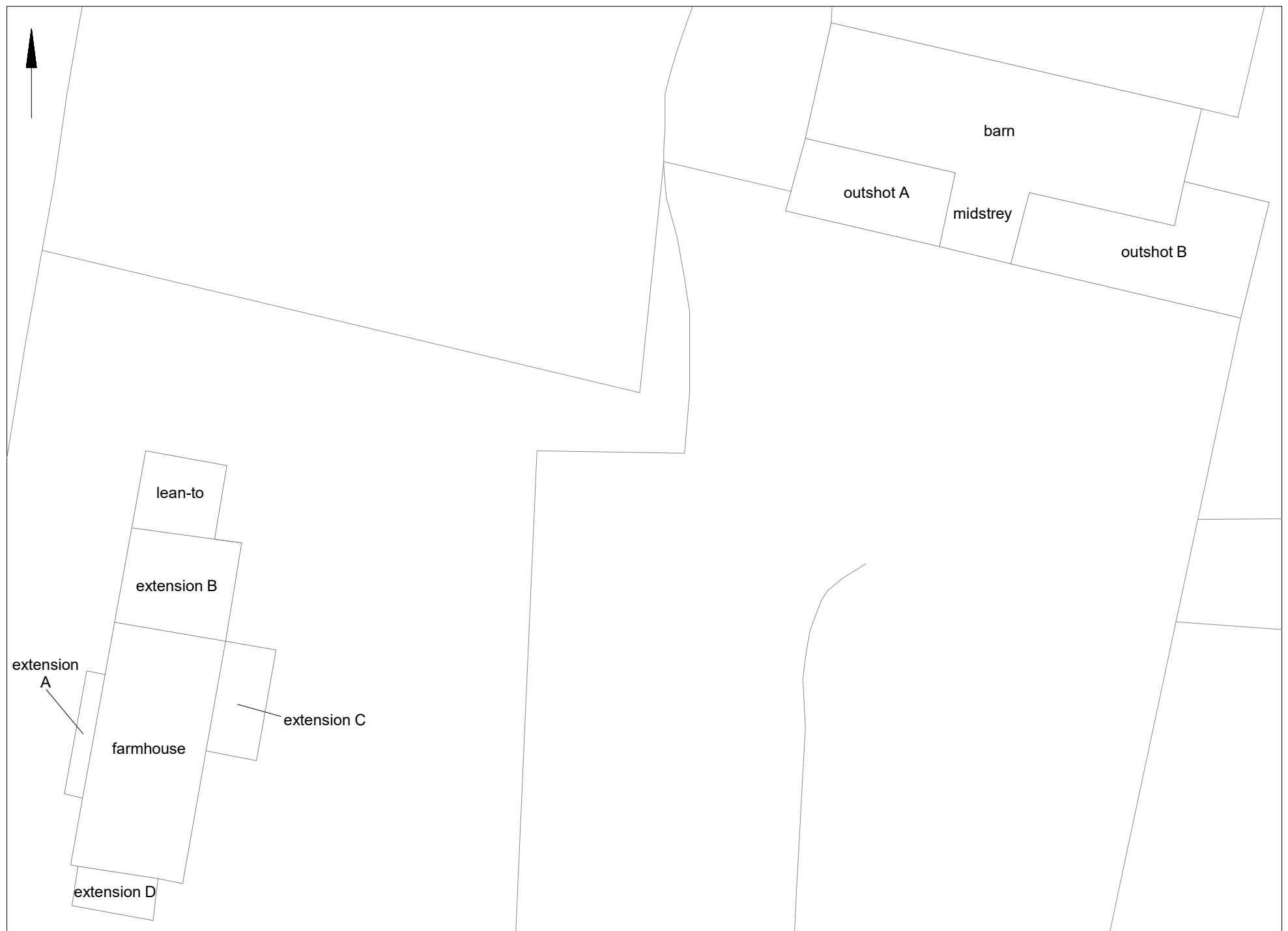
Fig 2 Detailed plan of site showing barn and farmhouse, with additions to the buildings labelled.
