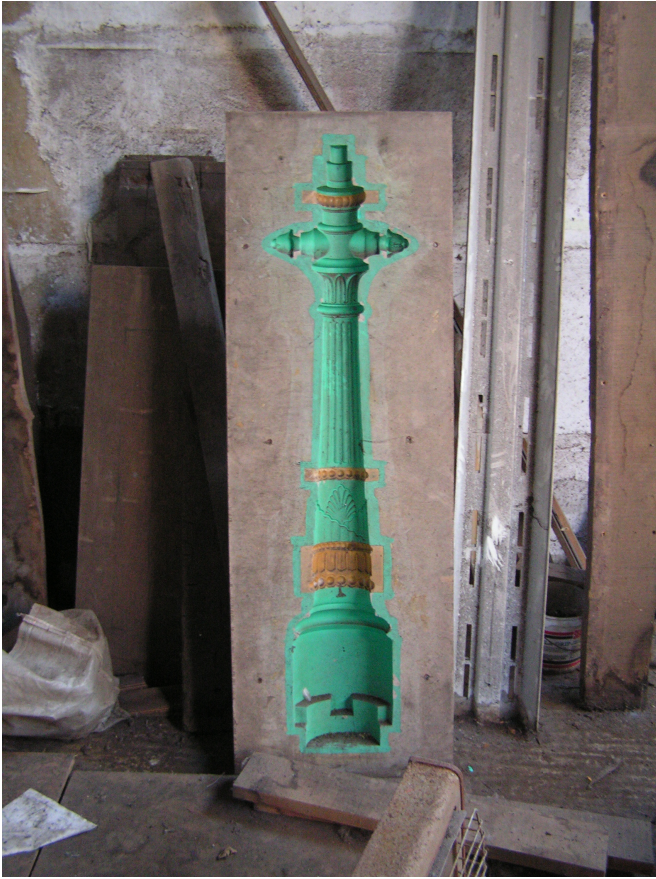
A1.5 Wooden pattern for bollard requiring a core, Building 3.
