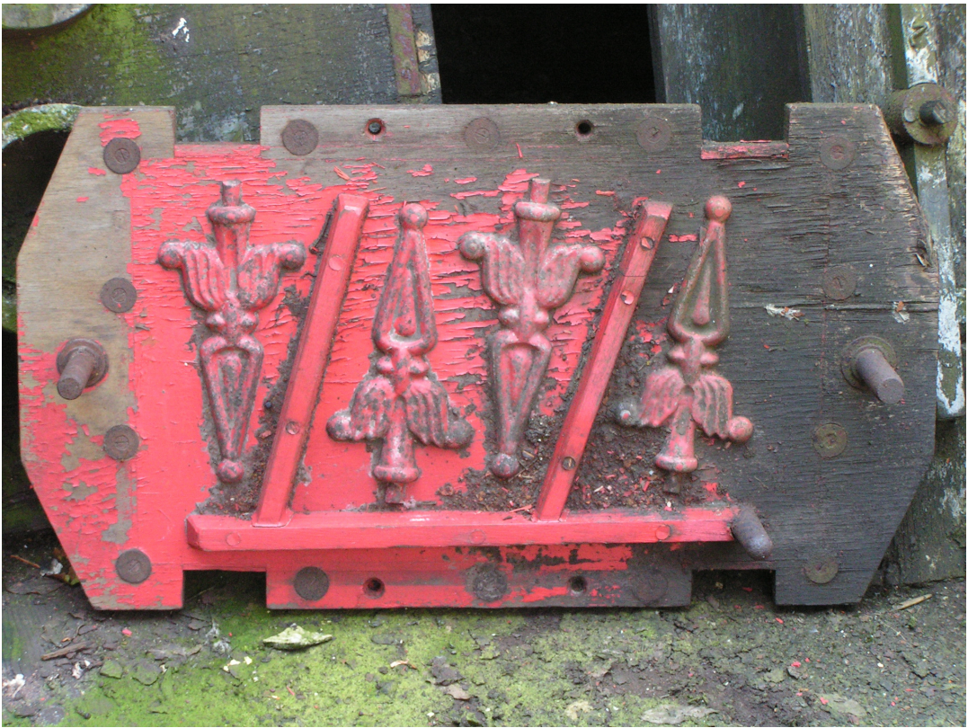
A1.6 Wooden pattern for ornamental railings, pattern loft.
