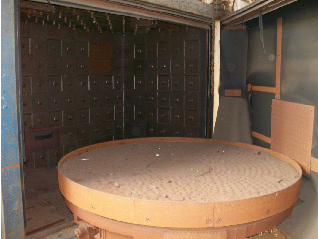
A1.19 Interior of Pangborn shot blasting machine, with blasting plate to the foreground, view north-west.
