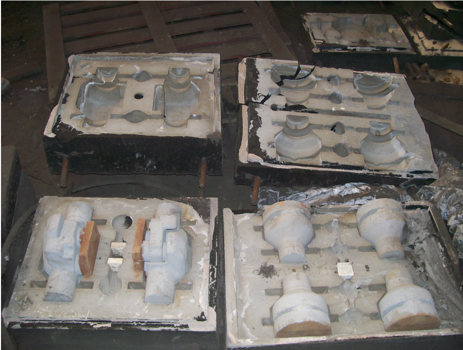
A1.11 Cores placed in moulds ready for casting.
