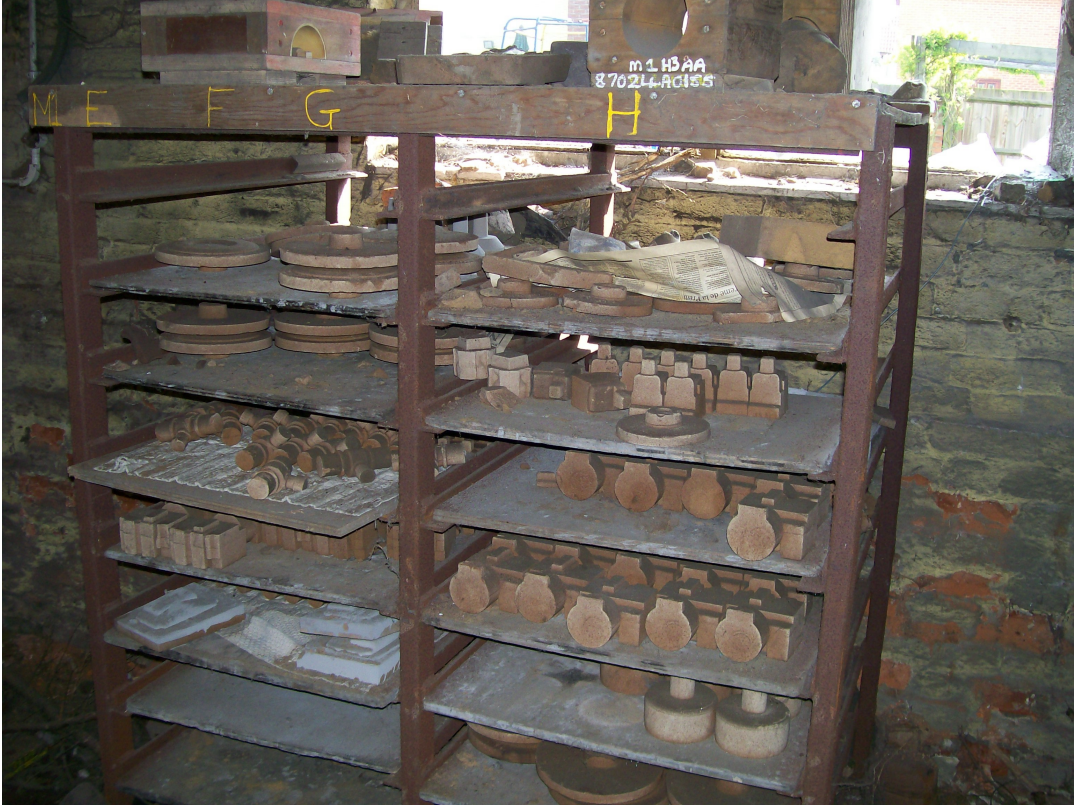
A1.8 Cores waiting to be baked in the core oven, view north-east.
