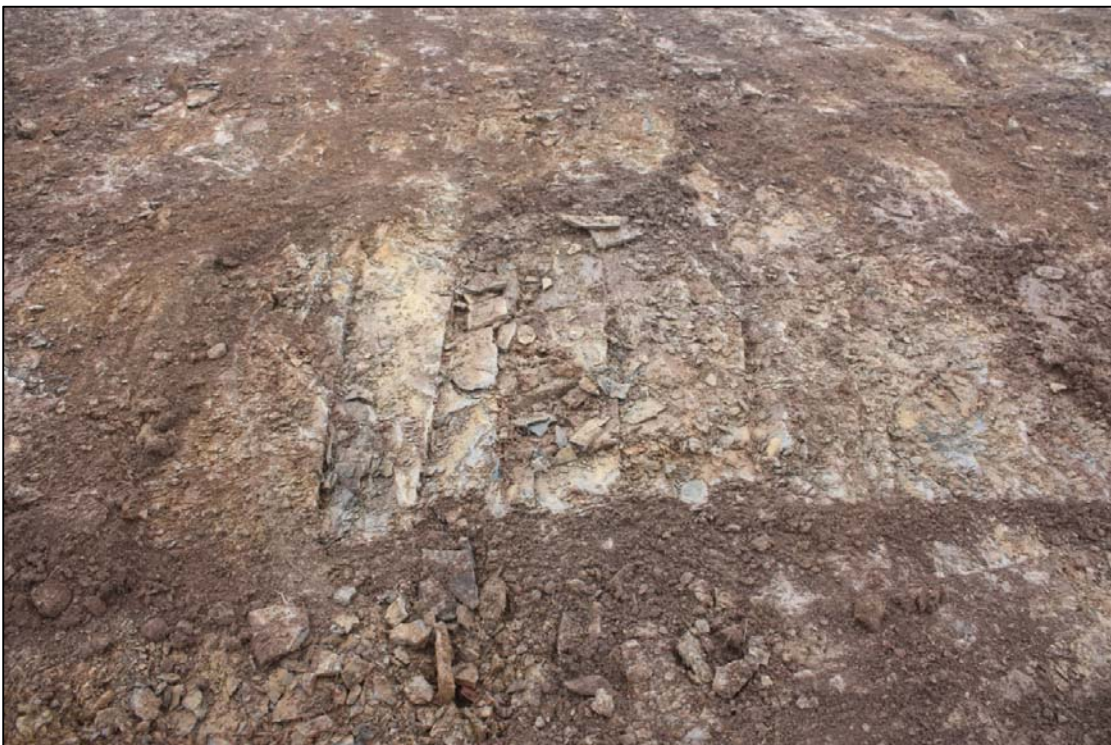
Photo 12 Typical chemically weathered bedrock over site
