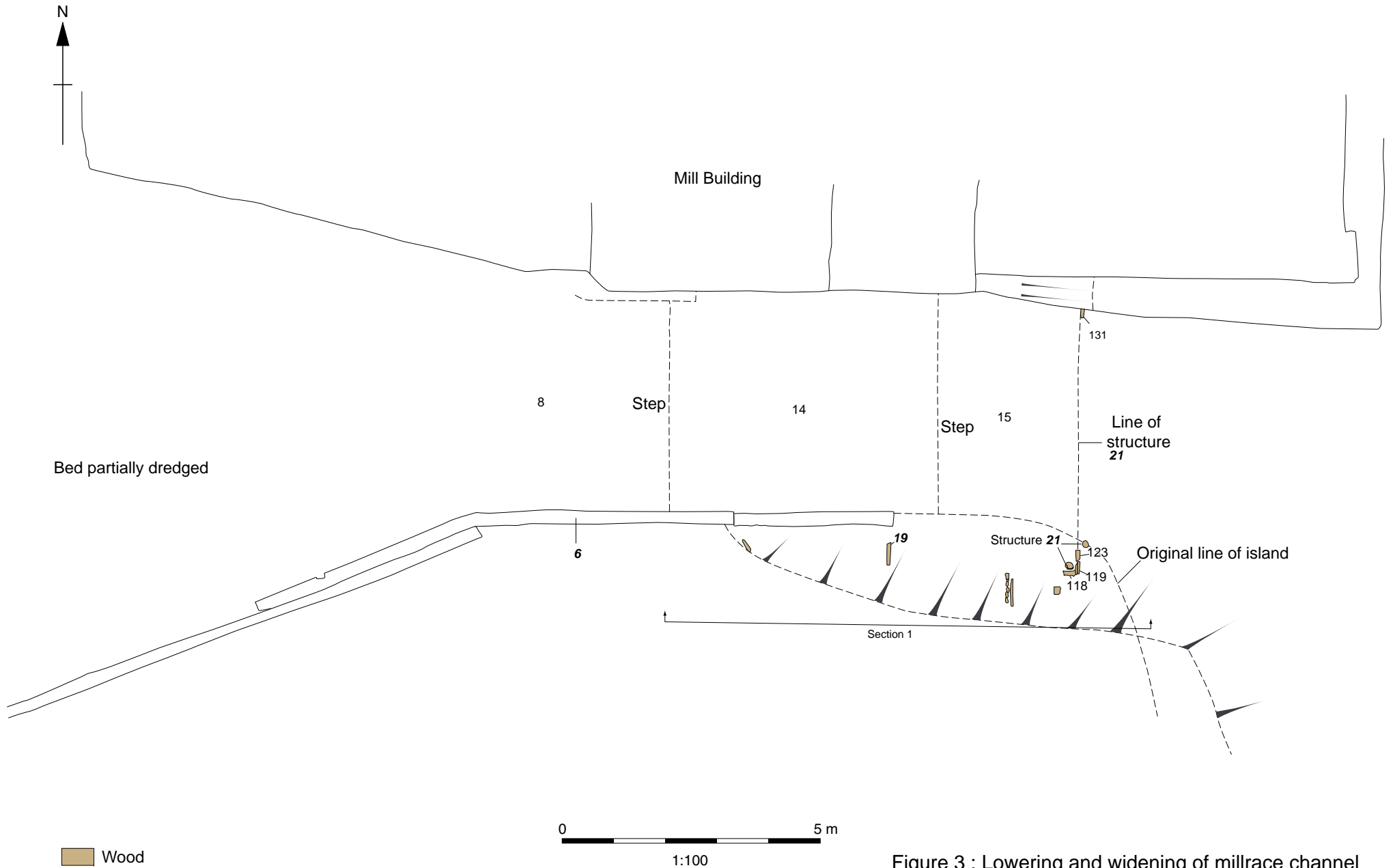
Figure 3 : Lowering and widening of millrace channel
